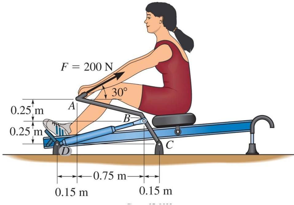
The woman exercises on the rowing machine. If she exerts a holding force of  $F = 200\text{ N}$  on the handle ABC, determine the reaction force at pin C and the force developed along the hydraulic cylinder BD on the handle.
