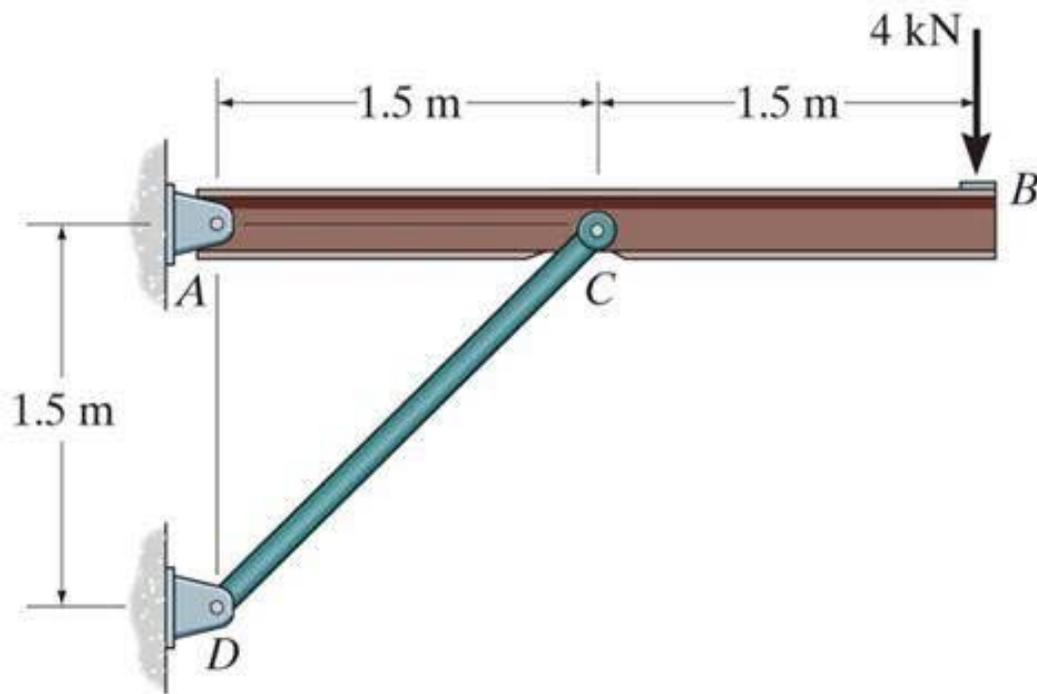
Given the 4kN load at B of the beam is supported by pins at A and C. Find the support reactions at A and C.
