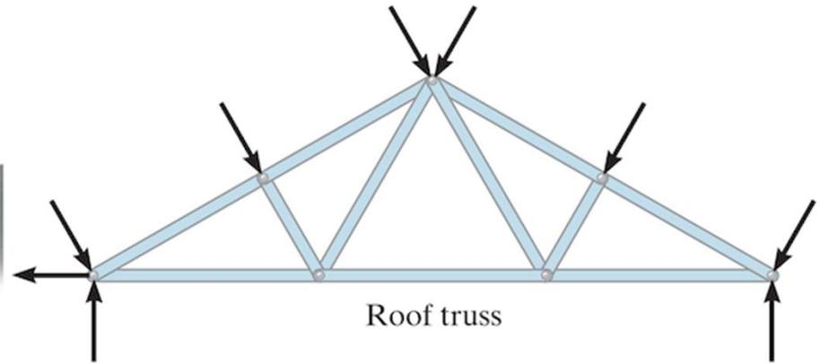
Load on roof transmitted to purlins, and from purlins to roof trusses at joints.
