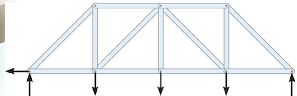
Load on deck transmitted to stringers, and from stringers to floor beams, and from floor beams to bridge trusses at joints.
