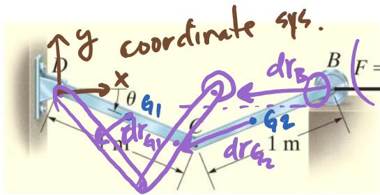
Determine the angle for equilibrium of the two-member linkage. Each member has a mass of 10 kg.
