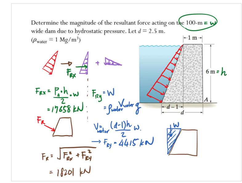
Determine the magnitude of the resultant force acting on on the 10-m wide dam due to hydrostatic pressure.
