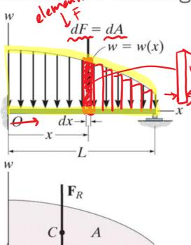
A common case of distributed loading in a uniform load along one axis of a flat rectangular body.
