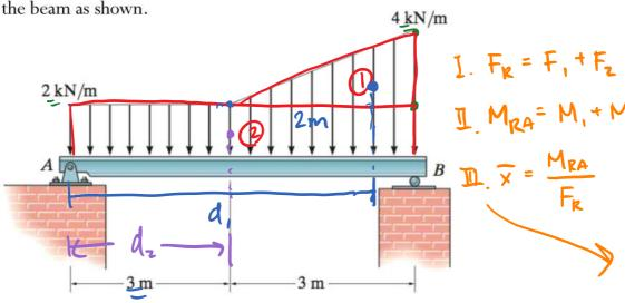
I.  $F_1 = \frac{1}{2}bh = \frac{1}{2}(3m)(4kN/m - 2kN/m) = 3kN$  $F_2 = bh = (6m)(2kN/m) = 12kN$
