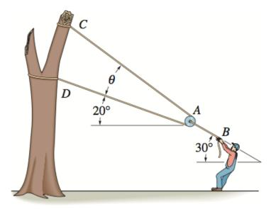
**Problem 7:** Determine the maximum weight of the crate that can be suspended from cables AB, AC, and AD so that the tension developed in any one of the cables does not exceed 250 lb. Draw the appropriate free-body diagram to solve this problem.
