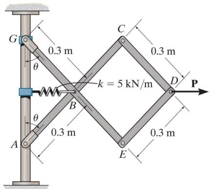
Determine the required force P needed to maintain equilibrium of the scissors linkage when the angle is 60 degrees. The spring is unstretched when the angle is 30 degrees.
