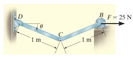
Determine the angle for equilibrium of the two-member linkage. Each member has a mass of 10 kg.
