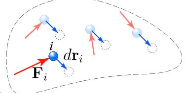
The work *dU* produced by the force *F* when it undergoes a differential displacement dr is given by
