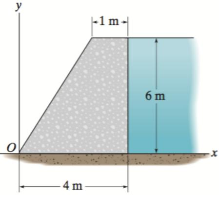
Determine the magnitude of the resultant force acting on on the 10-m wide dam due to hydrostatic pressure.
