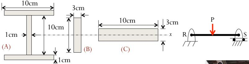
Consider three different possible cross sectional shapes and areas for the beam RS. For the given vertical loading P on the beam, which shape will develop less internal stress and deflection?
