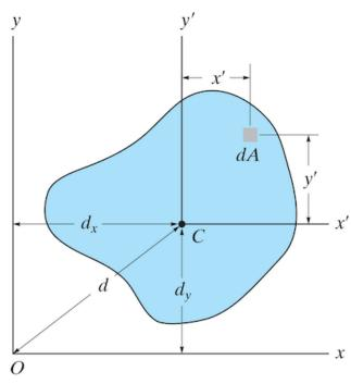
**Note:** the integral over y' gives zero when done through the centroid axis.
