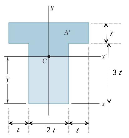
Determine the moment of inertia for the cross-sectional area about the *x* and *y* centroidal axes.
