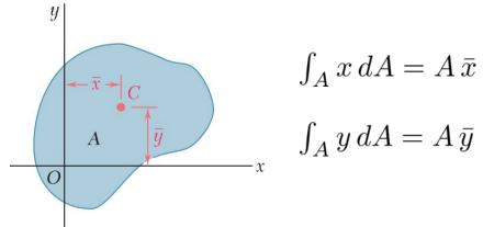
• In the case of a composite area, we divide the area A into parts
