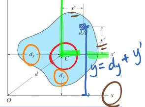
**Note:** the integral over y' gives zero when done through the centroid axis.
