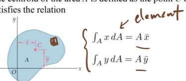
• In the case of a composite area, we divide the area A into parts
