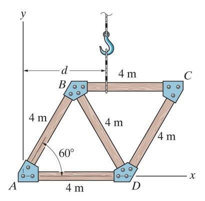
The truss is made from five members, each having a length of 4 m and a mass of 7 kg/m. Determine the distance *d* to where the hoisting cable must be attached, so that the truss does not tip (rotate) when it is lifted.
