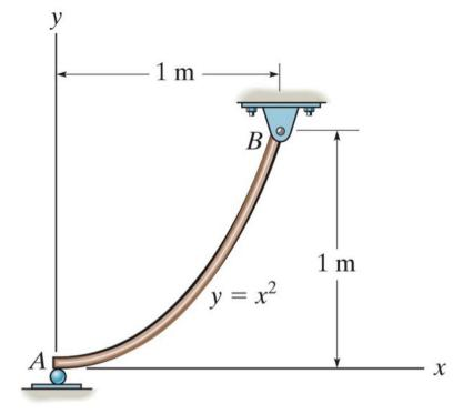
Locate the center of gravity  $\mathcal{X}$  of the homogeneous rod. If the rod has a weight per unit length of 100 N/m, determine the reaction supports at A and B.
