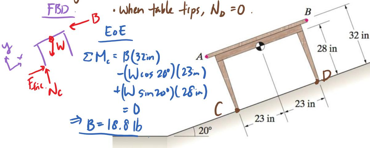
2.) Slipping Case: the most effective way is to push down the ramp at B as well.
