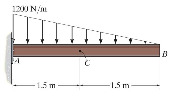
Draw the shear and moment diagrams for the cantilever beam.
