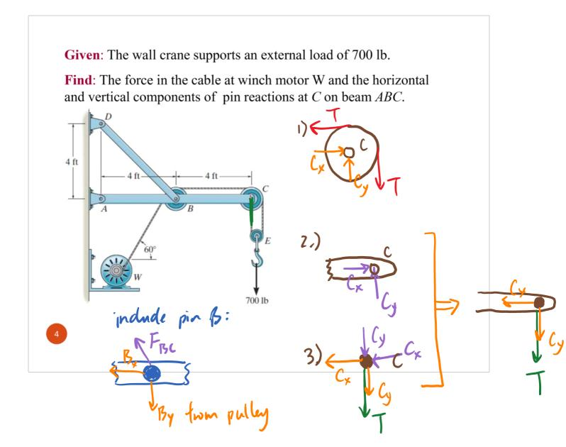
Determine the horizontal and vertical components of force which pin B exert on the frame.
