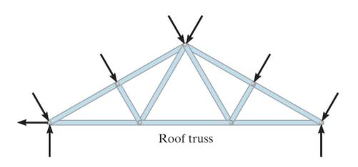
Load on roof transmitted to purlins, and from purlins to roof trusses at joints.
