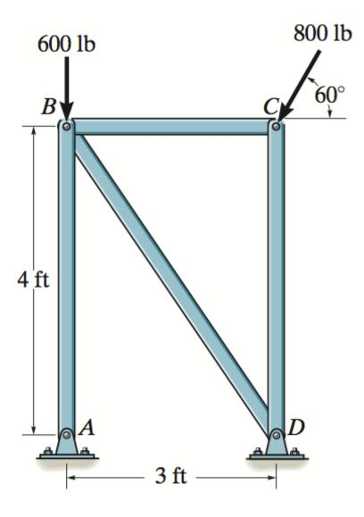
Find the forces in each member of the truss. Determine if members are in tension or compression.
