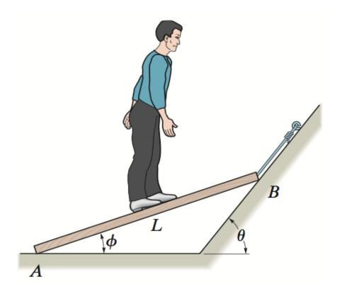
The uniform rod AB has a mass of 40 kg. Determine the force in the cable when the rod is in the position shown. There is a smooth collar at A.
