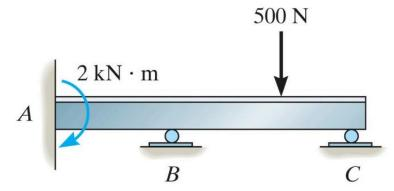
• Redundant constraints: the body has more supports than necessary to hold it in equilibrium; the problem is STATICALLY INDERTERMINATE and cannot be solved with statics alone
