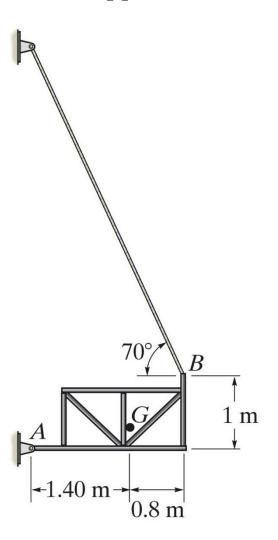
Determine the components of the support reactions at the fixed support *A* on the cantilevered beam.
