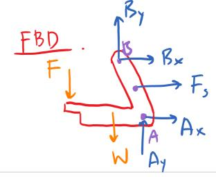
Find the tension in cable B given the weight of the cage.
