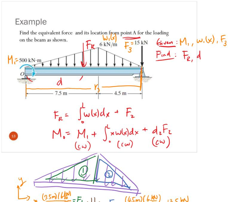
$\frac{(2.5m)(6\frac{kN}{m})}{2} = F_1 \quad \text{II} \quad F_2 = \frac{(4.5m)(6\frac{kN}{m})}{2} = 13.5 \text{ kN}$   $= 22.5 \text{ kN} \quad \text{F}_3 = \frac{(4.5m)(6\frac{kN}{m})}{2} = 13.5 \text{ kN}$   $= 22.5 \text{ kN} \quad \text{F}_4 = \frac{(4.5m)(6\frac{kN}{m})}{2} = 13.5 \text{ kN}$  = (22.5 + 13.5 + 15) kN  $M_A = Y_1 F_1 + Y_2 F_2 + Y_3 F_3 + M_1 \quad F_K = 51 \text{ kN}$  = (22.5 + 13.5 + 15) kN = (22.5 + 13.5 + 15) kN
