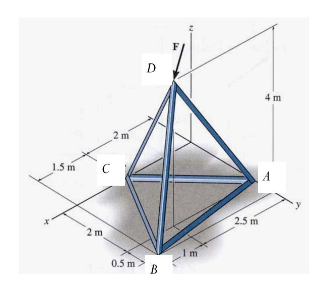
The force F = 10 N is acting along DC. Determine the moment of F about the bar BA.
