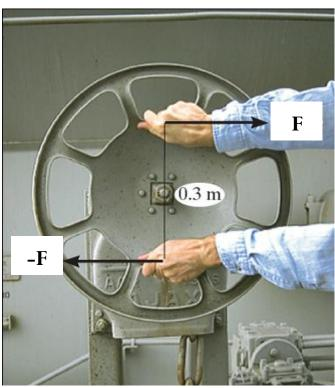
A torque or moment of 12 N·m is required to rotate the wheel. Would F be greater or less than 30 N?
