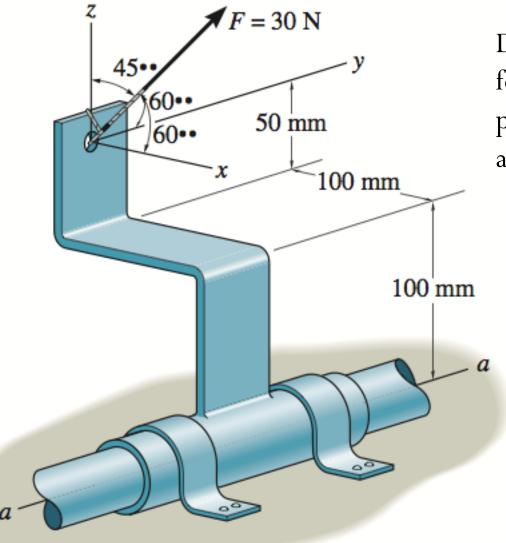
Determine the moment of the force about the a-a axis of the pipe. ( $\alpha = 60^{\circ}$ ,  $\beta = 60^{\circ}$ , and  $\gamma = 45^{\circ}$ )
