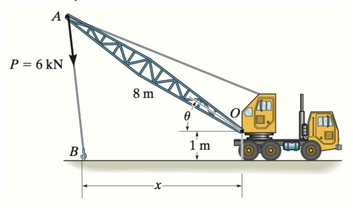
**Given:** The angle  $\theta = 30^{\circ}$  and x = 10 m.
