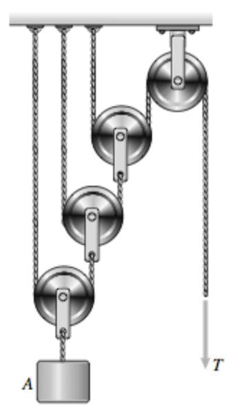
The mass of the suspended object A is  $m_A$  and assume the masses of all pulleys are negligible, determine the force T necessary for the system to be in equilibrium.
