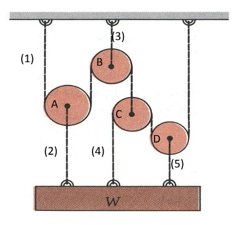
The five ropes can each take 1500 N without breaking. How heavy can W be without breaking any?
