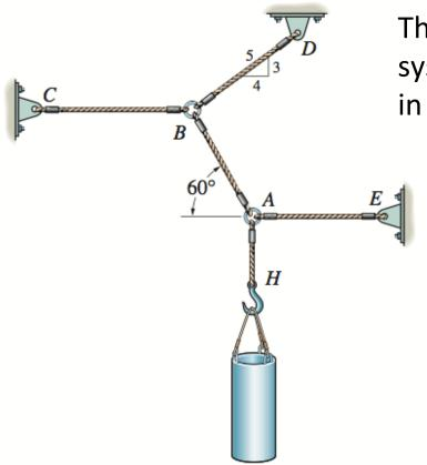
The 30-kg pipe is supported at A by a system of five cords. Determine the force in each cord for equilibrium.
