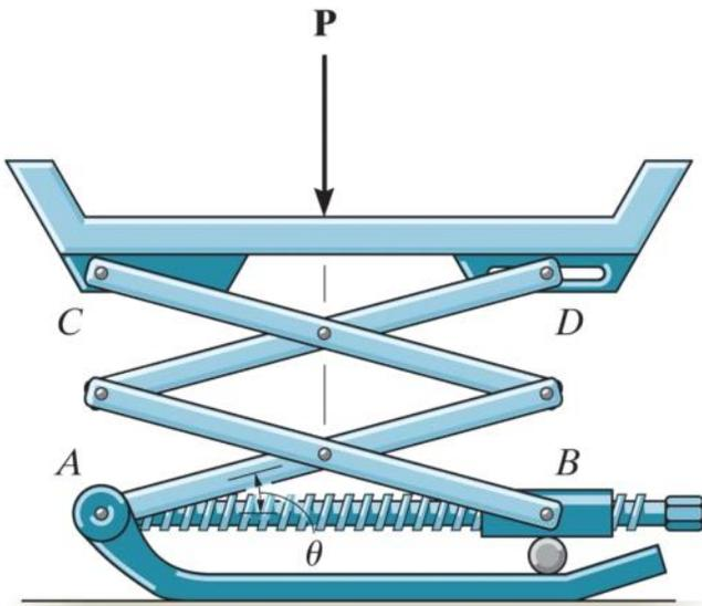
The scissors jack supports a load  $P$ . Determine the axial force in the screw necessary for equilibrium when the jack is in the position  $\theta$ .
