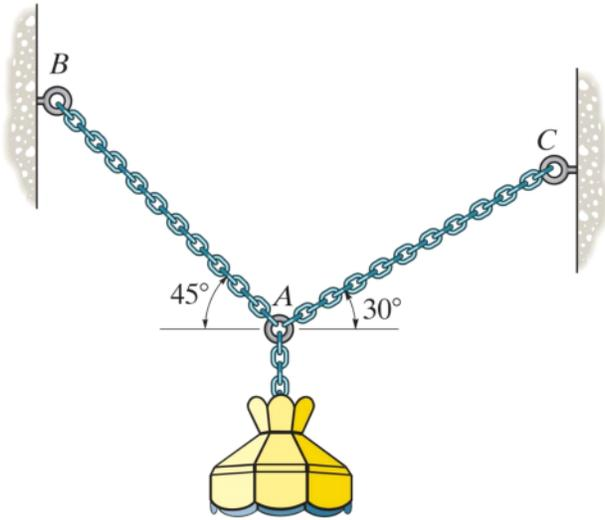
Determine the tension in the cable AC. The lamp weighs 10 lb.
