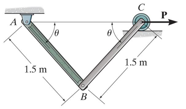
Determine the required magnitude of force P to maintain equilibrium of the linkage at an angle of 60 degrees. Each member has a mass of 20 kg.
