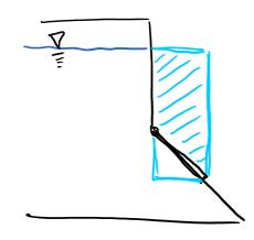
the horizontal component is the same as above. the vertical component is the weight of "WATER" About the GATE.
