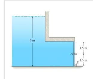
The 2-m-wide rectangular gate is pinned at its center A and is prevented from rotating by the block at B. Determine the reactions at these supports due to hydrostatic pressure.
