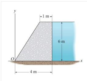
The factor of safety for tipping of the concrete dam is defined as the ratio of the stabilizing moment due to the dam's weight divided by the overturning moment about O due to the water pressure. Determine this factor if the concrete has a density of  $2500 \, \text{kg/m}^3$ .
