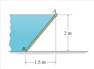
Determine the magnitude of the hydrostatic force acting on gate AB which has a width of 1.5 m.
