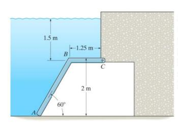
Determine the magnitude of the resultant force acting on the gate ABC due to hydrostatic pressure. The gate has a width of 1.5 m and the density of the water is 1000 kg/m<sup>3</sup>.
