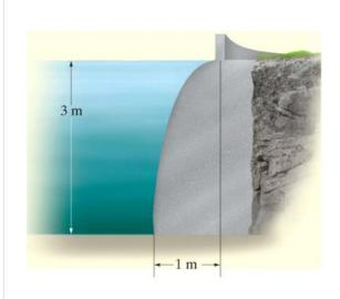
Determine the magnitude and location of the resultant hydrostatic force acting on the surface of a seawall shaped in the form of a parabola. The wall is 5 m. The density of the sea water is  $1020 \, \text{kg/m}^3$
