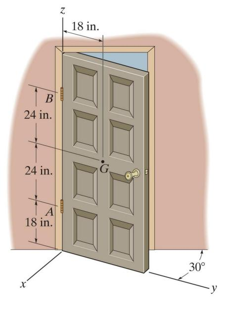
The 100 lb door has its center of gravity at *G*. Determine the components of reaction at hinges *A* and *B* if hinge B resists only forces in the x and y directions and A resists forces in the x, y, z directions.
