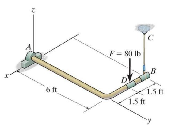
Given: The rod, supported by thrust bearing at A and cable BC, is subjected to an 80 lb force.
