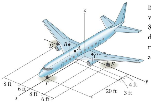
If these components have weights  $W_A = 45000$  lb,  $W_B = 8000$  lb and  $W_C = 6000$  lb, determine the normal reactions of the wheels D, E, and F on the ground.
