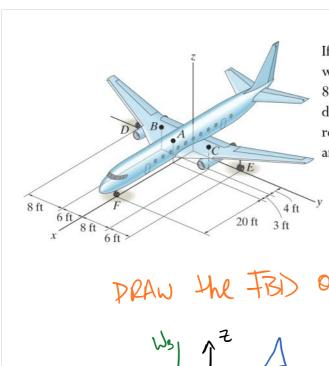
If these components have weights  $W_A = 45000$  lb,  $W_B =$ 8000 lb and  $W_C = 6000$  lb, determine the normal reactions of the wheels D, E, and F on the ground.
