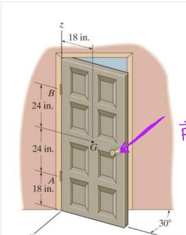
The 100 lb door has its center of gravity at G. Determine the components of reaction at hinges A and B if hinge B resists only forces in the x and y directions and A resists forces in the x, y, z directions.
