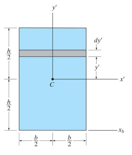
Determine the moment of inertia for the rectangular area shown w.r.t. the centroidal axis x'.
