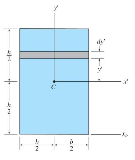
Determine the moment of inertia for the rectangular area shown w.r.t. the axis passing through the base of the rectangle  $x_b$ .
