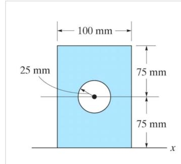
Determine the moment of inertia for the shaded area about the *x* axis.
