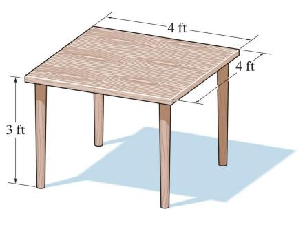
The wooden table is made from a square board having a weight of 15 lb. Each of the legs weighs 2 lb and is 3 ft long.
