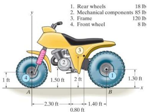
Determine the location of the center of gravity of the three-wheeler. If the three-wheeler is symmetrical with respect to the x-y plane, determine the normal reaction each of its wheels exerts on the ground.
