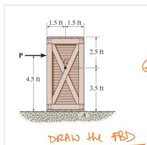
Find the maximum force P that can be applied without causing movement of the crate.
