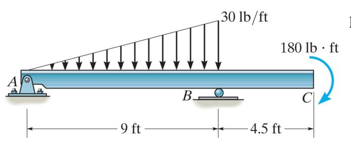
Draw the shear and moment diagrams for the beam.
