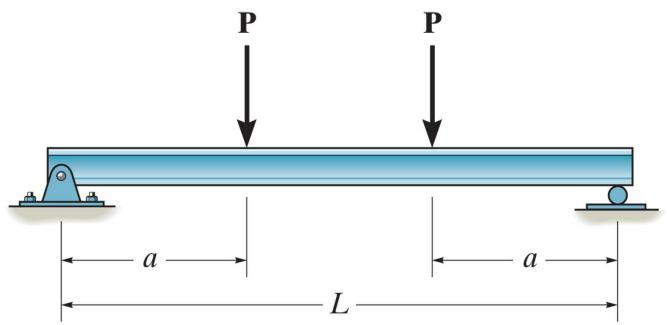
Draw the shear and moment diagrams for the beam.
