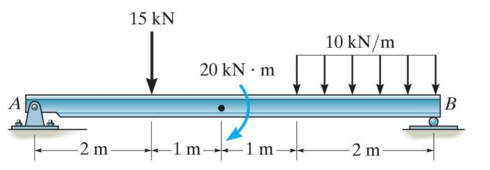
Draw the shear and moment diagrams for the beam.
