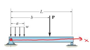
Draw the shear and moment diagrams for the simply supported beam.
