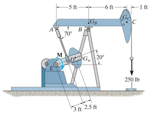
The pumping unit is used to recover oil. Determine the torque **M** which must be exerted by the motor in order to overcome this load.
