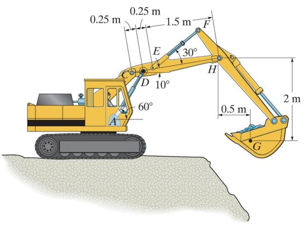
Determine the force created in the hydraulic cylinders EF and AD in order to hold the shovel in equilibrium. The shovel load had a mass of 1.25 Mg and center of gravity at G.
