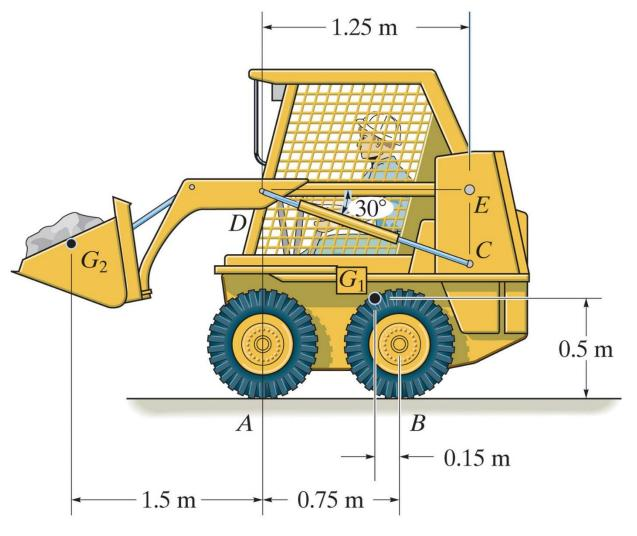
Determine the reactions of each pair of wheels A and B on the ground and the force in the hydraulic cylinder CD and at the pin E.
