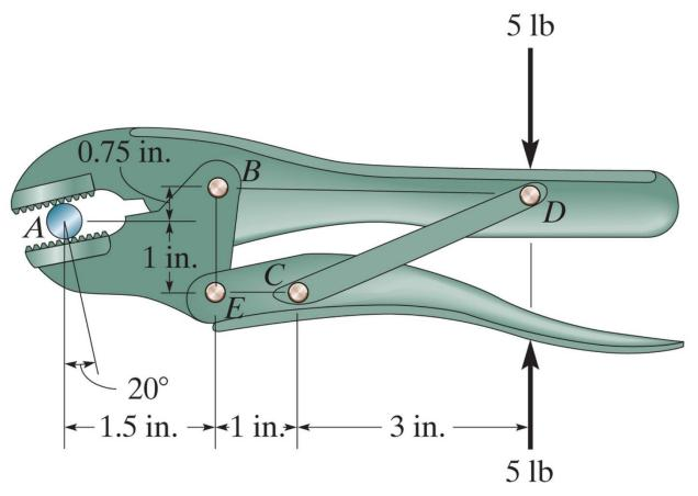
A 5 lb force is applied to the handles. Determine the compressive force developed at the smooth bolt shank A at the jaws.
