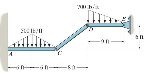
Determine the reactions at supports A and B.
