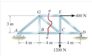
Determine the force in member GC and GE of the truss and state if the members are in tension or compression.
