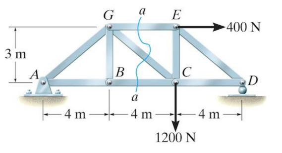
Determine the force in member GC and GE of the truss and state if the members are in tension or compression.
