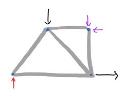
In  $\equiv$ M, the truss is A rigid structure, Composed of rigid members, connected by smooth pins. for A given configuration And External landing, Members experience tension or compression.
