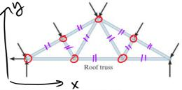
Load on roof transmitted to purlins, and from purlins to roof trusses at joints.
