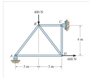
Find the forces in each member of the truss. Determine if members are in tension or compression.
