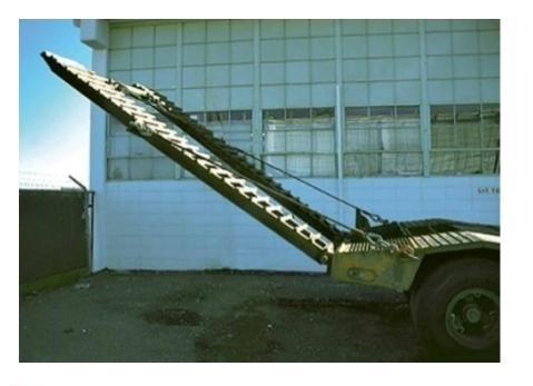
The uniform truck ramp has weight 400 lb and is pinned to the body of the truck at each side and held in the position shown by the two side cables. Determine the reaction forces at the pins and the tension in the cables.
