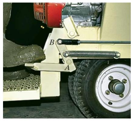
The operator applies a vertical force to the pedal so that the spring is stretched 1.5 in. and the force in the short link at B is 20 lb. Determine the vertical force applied to the pedal.
