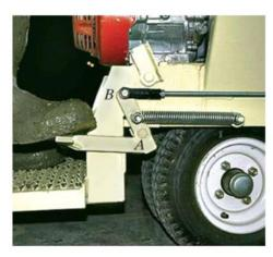
The operator applies a vertical force to the pedal so that the spring is stretched 1.5 in. and the force in the short link at B is 20 lb. Determine the vertical force applied to the pedal.
