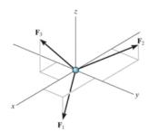
In contrast to the forces on a particle, the forces on a rigid-body are not usually concurrent and may cause rotation of the body.
