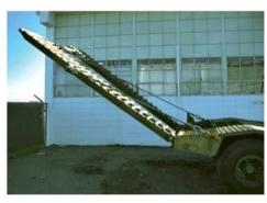
The uniform truck ramp has weight 400 lb and is pinned to the body of the truck at each side and held in the position shown by the two side cables. Determine the reaction forces at the pins and the tension in the cables.
