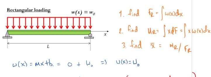
$$\overline{M}_{e} = \int_{0}^{L} x dF = \int_{0}^{L} w_{o} x dx = w_{o} \left[\frac{x^{2}}{z}\right]_{0}^{L} = \frac{1}{z} w_{o} L^{2}$$
