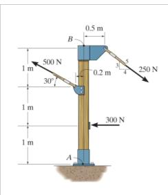
Replace the force system acting on the post by a resultant force and resultant moment about point A, and specify where its line of action intersects the post AB measured from point A.
