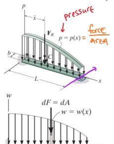
In structural analysis, we often are presented with a **distributed load** w(x) (force/unit length) and we need to find the equivalent loading F.
