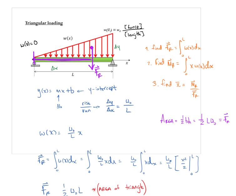
$$\overrightarrow{M}_{R} = \int_{-\infty}^{L} x \omega(x) dx = \int_{-\infty}^{L} \frac{\omega_{0}}{x^{2}} x^{2} dx = \frac{\omega_{0}}{L} \int_{0}^{L} x^{3} dx = \frac{\omega_{0}}{L} \left[ \frac{x^{3}}{3} \right]_{0}^{L}$$
