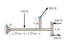
Replace the force and couple system acting on the member by an equivalent force and couple moment acting at point O.
