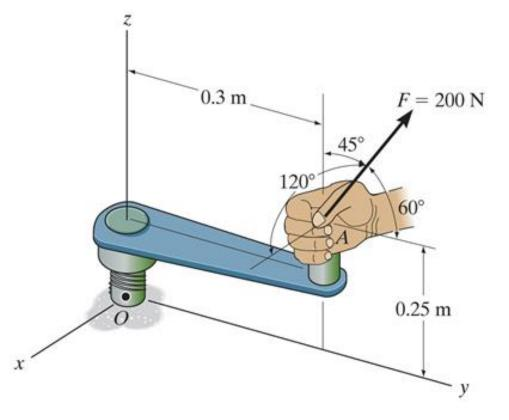
A force is applied to the tool as shown. Find the magnitude of the moment of this force about the x axis of the value.
