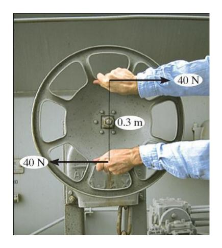
A torque or moment of 12 N·m is required to rotate the wheel. Why does one of the two grips of the wheel above require less force to rotate the wheel?
