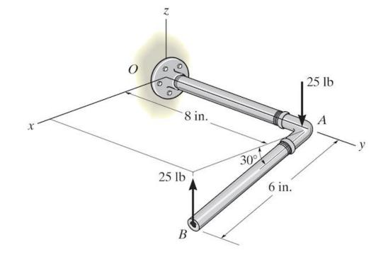
Determine the moment acting on the pipe about O.
