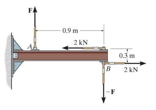
Two couples act on the beam with the geometry shown. Find the magnitude of F so that the resultant couple moment is 1.5 kN·m clockwise.
