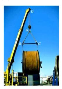
For a spool of given weight, how would you find the forces in cables AB and AC? If designing a spreader bar (BC) like this one, you need to know the forces to make sure the rigging (A) doesn't fail.
