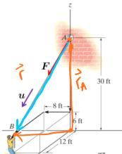
The force vector  $\mathbf{F}$  acting a long the rope can be defined by the unit vector  $\boldsymbol{u}$  (defined the <u>direction</u> of the rope) and the
