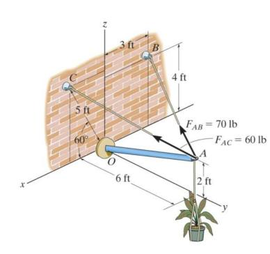
Determine the projected component of the force vector  $F_{AC}$  along the axis of strut AO. Express your result as a Cartesian vector
