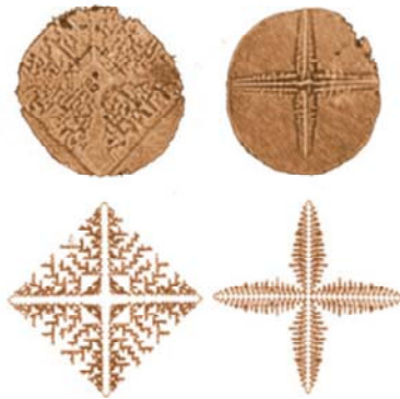
→ Figure 6. Microphotographic images of pressure-induced dendritic crystals (top row) are remarkably similar to the patterns produced in computer simulations of temperature-driven dendritic crystal growth (bottom row). [1] (Courtesy Lawrence Livermore National Laboratory)
