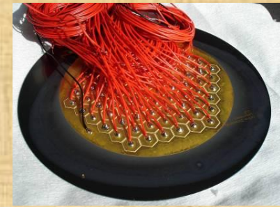
Soldered control and mass wires
