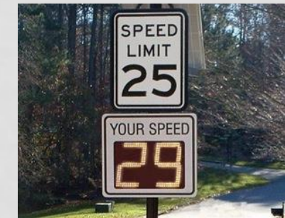
Motion detector (10.4GHz)
