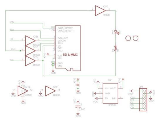
For the level shifter we use the CD74HC4050 which has a typical propagation delay of ~10ns
